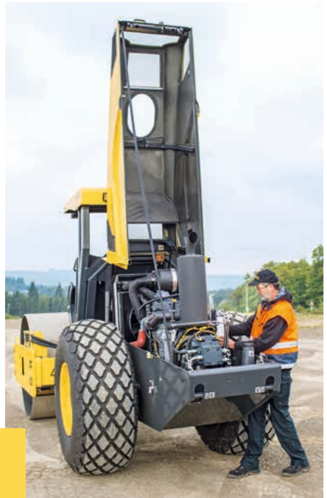
Easy Service: no grease nipples on the -40 single drum rollers.
